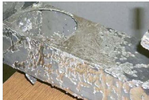
Wave pot assembly erosion
