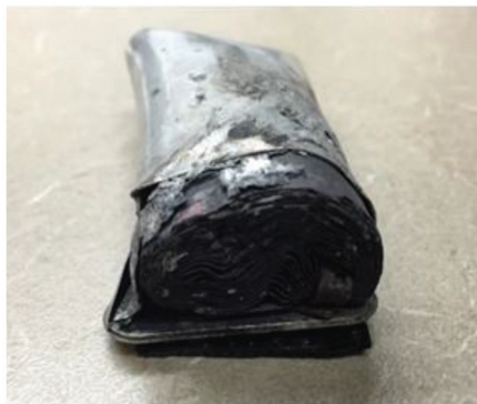
After thermal runaway
