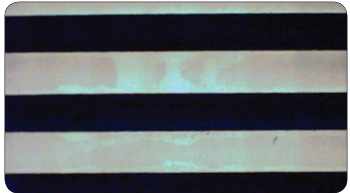
Figure 18. Example of a passing SIR board, backlight, 30X mag.
