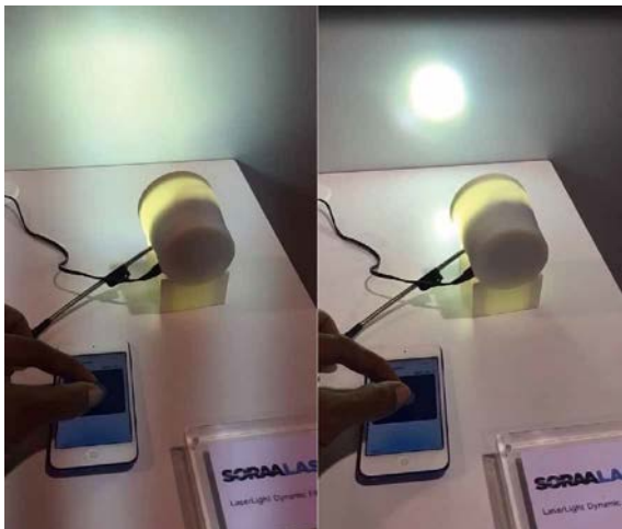
Figure 6: Dynamic control of the beam angle with an LC lens operated by a touchpad
