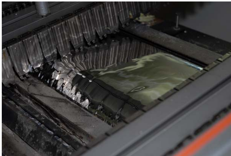
Figure 13, Low dross formed with SnCu based solder
