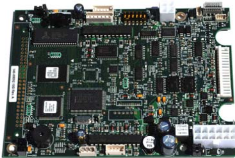
Figure9. ENIG board with lead-free parts soldered
