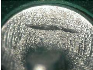
Figure2. SAC hot tear
