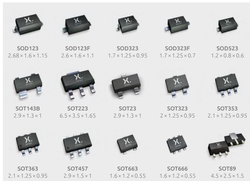
Figure 92 | Table of Nexperia diode leaded-packages with outline and dimensions in mm.
